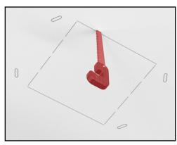
2. Place the drywall bracket to the side and cut out the marked square using a jab saw.
