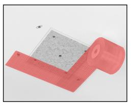
12. Tape the seams between the drywall board and ceiling. Joint compound may be used to fill any gaps before applying the tape.
