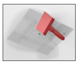
13. Allow for the tape to dry and apply your first coat of plaster to the tape seam, lightly skim coating the surface of the fixture board assembly.
