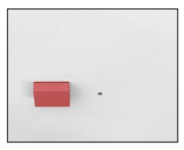
15. Wait until the surface has fully dried, and sand the plastered ceiling to match the surrounding level of drywall.
