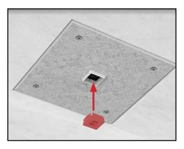
**9.** Insert the finishing guard into the fixture opening to prepare for finishing. The fixture must remain off for the remainder of the installation.
