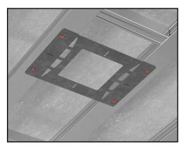
**1.** Separate the mounting bracket and mounting board and fasten the bracket to the framing in the desired fixture location.
