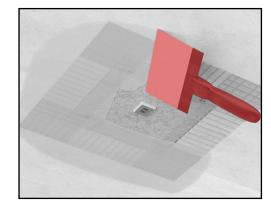
**11.** Allow for the tape to dry and apply your first coat of plaster to the tape seam, lightly skim coating the surface of the fixture board assembly.
