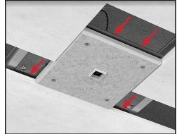
8. Cut and install the drywall around the fixture, ensuring that the fixture board assembly is flush with the surrounding drywall. This will allow a finish of one eight inch of plaster around the finishing guard.
