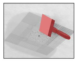
10. Allow for the tape to dry and apply your first coat of plaster to the tape seam, lightly skim coating the surface of the fixture board assembly.
