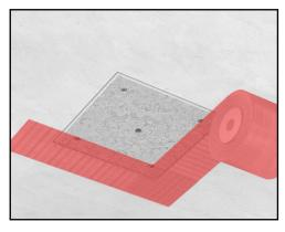
9. Tape the seams between the drywall board and ceiling. Joint compound may be used to fill any gaps before applying the tape.
