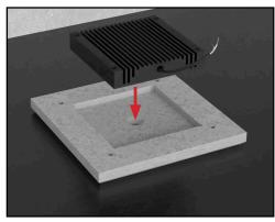
2. Take the Minus fixture and place it onto the mounting board.
