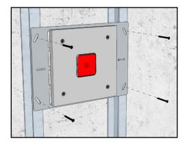
**2.** Fasten the bracket to the framing using the screws provided with the bracket.
