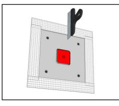
**9.** Tape the seams between the drywall board and ceiling. Joint compound may be used to fill any gaps before applying the tape. Allow for the tape to dry and apply your first coat of plaster to the tape seam.
