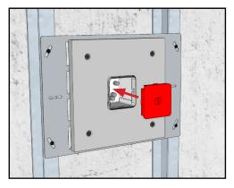
**7.** Safely remove the fixture and insert the finishing guard into the fixture opening to prepare for finishing.
