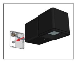
13. Make the low voltage electrical connection.
