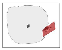
7. Allow for the tape to dry and apply your first coat of plaster to the tape seam, lightly skim coating the surface of the fixture board assembly.
