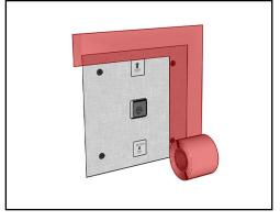
6. Tape the seams between the drywall board and ceiling. Joint compound may be used to fill any gaps before applying the tape.
