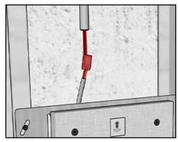
2. Feed low voltage wiring to the fixture board assembly and make the low voltage connection.
