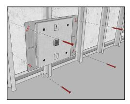
1. Fasten the bracket to the framing in the desired fixture location. Insure that the "TOP" label is facing towards the ceiling and the "DOWN" label is facing towards the floor.
