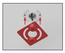
7. Take the installation bracket and secure it to the ceiling with the appropriate hardware.
