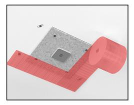
**13.** Tape the seams between the drywall board and ceiling. Joint compound may be used to fill any gaps before applying the tape.
