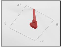
**2.** Place the drywall bracket to the side and cut out the marked square using a jab saw.
