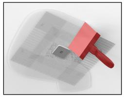
**14.** Allow for the tape to dry and apply your first coat of plaster to the tape seam, lightly skim coating the surface of the fixture board assembly.
