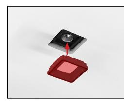
**19.** Insert the louver into the fixture opening to magnetically attach the louver.
