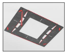
**1.** Ensure that any existing framing or studs do not interfere with the intended fixture location. Using the bracket as a template, mark the drill and cut lines with a pencil. The bracket has center lines to help with the alignment of the fixture.
